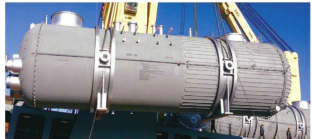
Project Shah Gas Develop.(SGD) & U.A.E Dimension 5,900ID x 19,800L, 375Ton Equipment Sulphur Condenser
